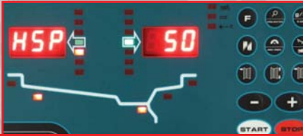
Easy identification of ALU mode with bright LEDs indicating selected weight position
