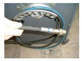
3. The system should also be connected to a compressed air line
