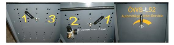
valve set to "3-2" (lever right and left) empties the new oil tank.
