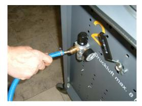
(Set pressure reducer to 8 bar), so that automatic motor running recognition and oil return flow are possible.
