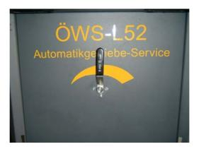
11. When the waste oil reaches the mark, set the right setting lever to "3". The oil now circulates in the new oil tank. The oil change is now completed.
